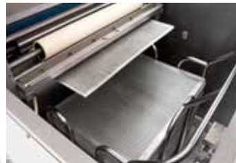
The trays are fed through the unique brush system directly into the receiving section and from there to the receiving tray wagon.
