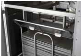
A vacuum system operating with pneumatics lifts the tray from the tray wagon using four suction pads and feeds it into the tray cleaner system.
