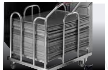
When the system stops, the tray wagon containing the clean trays is removed and an empty wagon can be put into place. The system is now able to continue cleaning more trays.
