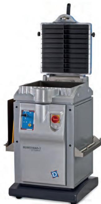
Daub's Robotrad-t is a hydraulic divider for artisan bread that benefited from a long pre-proofing time. By using a grill inside the lid, it is possible to divide the dough without the use of any pressure. Dividing is achieved by pushing the dough against the removable grill which is available in various long, square and triangle versions.
