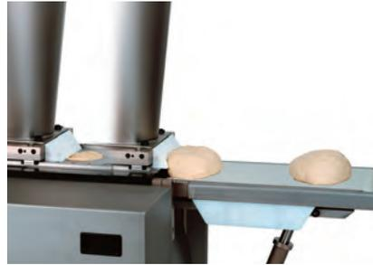
Vacuum scaling system with built-in vacuum pump.
