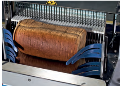
Cutting blades are constructed in a strong and solid frame module.
