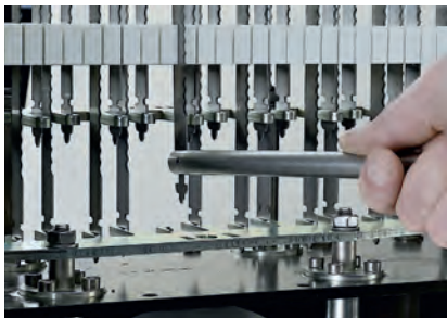
Replacement of teflon coated blades within seconds without need of a service technician.
