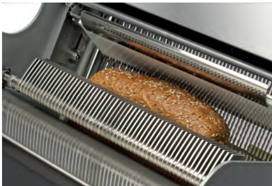
Slicing blades are constructed in a strong and solid frame module for smooth and silent slicing.
